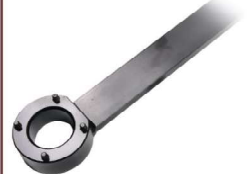
CRANKSHAFT PULLEY HOLDER Holds vibration damper when loosening and tightening center crankshaft bolt. Suitable engines: VAG 1.8L & 2.0L TFSI / TSI 2008→ OEM code: T10355
